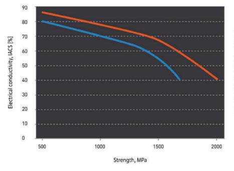
The figure shows the range of values of the combination of strength and electrical conductivity of niobium copper-based nanocomposite wires. The upper red curve limits the field for achieving the maximum achieved values of the combination of strength and electrical conductivity of such wires. The lower blue curve characterizes the normally achieved level of combination of these values.
