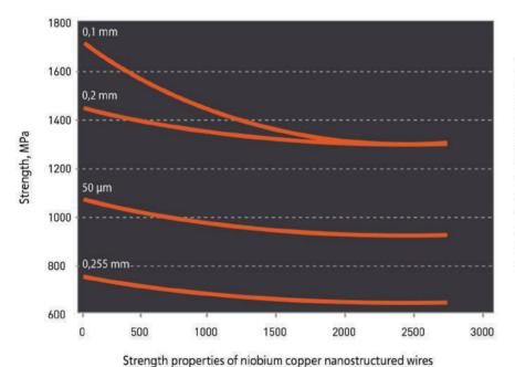
The curves shown in the graph demonstrate the strength properties of nanostructured conductors of 0.1 mm, 0.2 mm, 50 µm, and 0.255 mm in diameter during tests at 350°C. The graph illustrates the high stability of niobium copper-based nanostructured materials strength properties. The strength of thin and fine conductors exceeds the strength properties of conventional electrical wires significantly even after 2,660 hours of exposure at 350°C.
