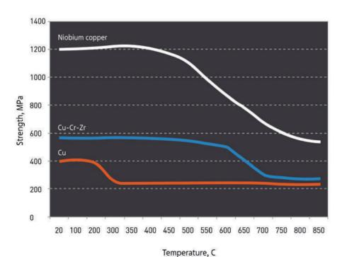
Nanocomposite wires have mechanical strength comparable to steel (1200-1500 MPa). Their electrical conductivity level reaches 70-85% of the absolute electrical conductivity characteristic of pure copper. The technical process of nanocomposite wires production is currently considered unique in Russia and worldwide and allows to manufacture wires of any diameters and cross sections from innovative material.
